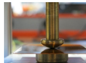
Figure 3. Dielectric strength measuring setup
